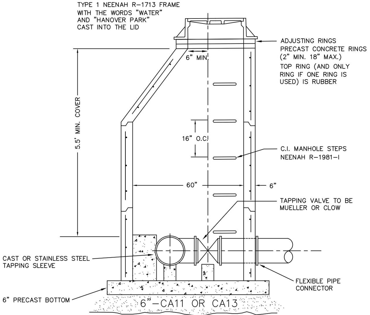
PRE-CAST REINFORCED CONCRETE RISER RINGS AND DOMES SHALL COMPLY WITH ASTM C-39.
