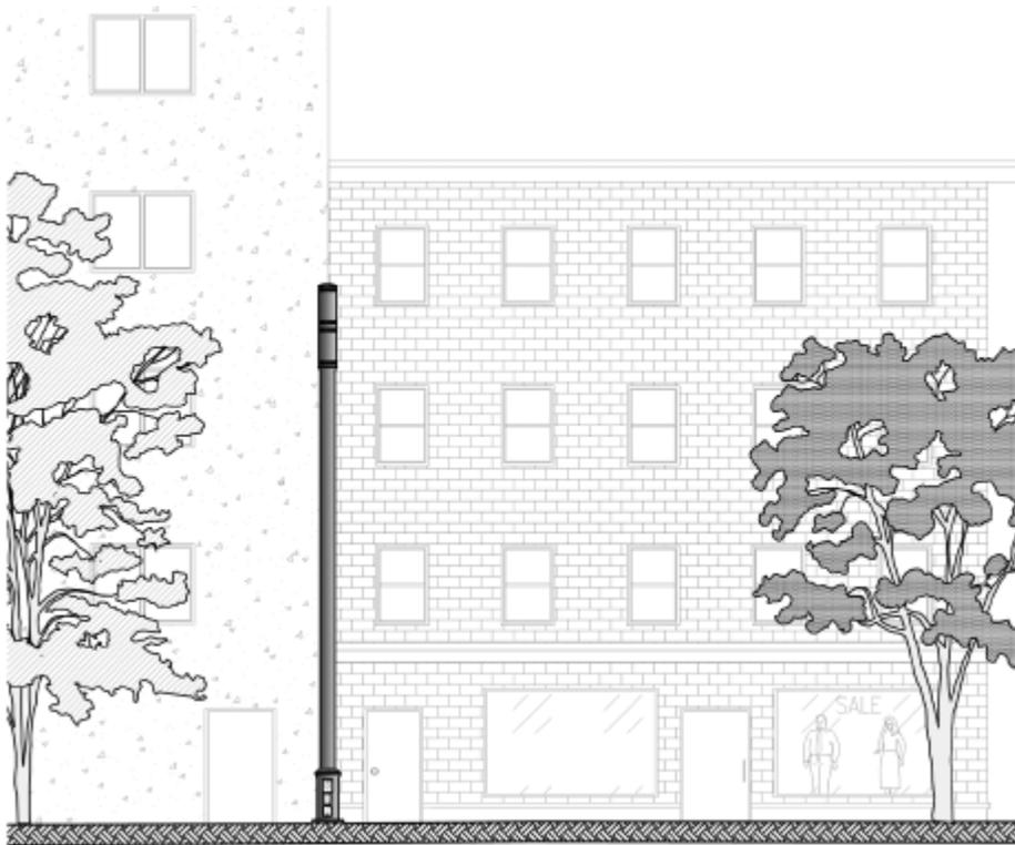
When located adjacent to a commercial establishment, such as a shop or restaurant, care should be taken to locate the small cell such that it does not negatively impact the business. Small cells shall not be located in-front of store front windows, primary walkways, primary entrances or exits, or in such a way that it would impede a delivery to the building. Small cells should be located between properties as much as possible as shown in Figure 6.
