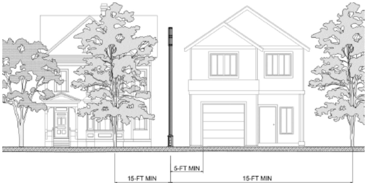
Freestanding small cells shall be located at intersecting property lines as much as possible. Whenever possible, the freestanding small cell shall be located on the secondary street. Small cells shall also be located a minimum of 15 feet away from trees to prevent disturbance within the critical root zone of any tree, as shown in Figure 4.
