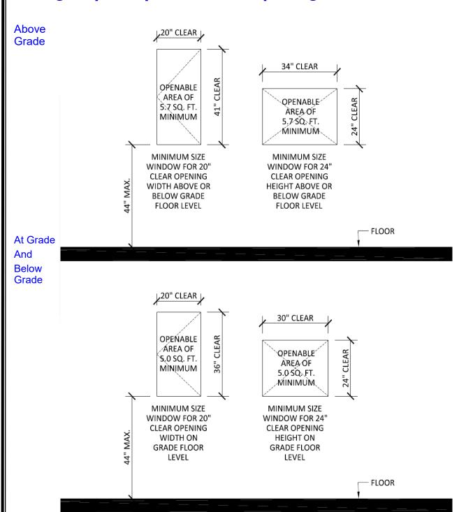
NOTE: WINDOW WELLS SHALL HAVE A MINIMUM HORIZONTAL AREA OF 9 SQ. FT. WITH A MINIMUM HORIZONTAL PROJECTION AND WIDTH OF 36"
